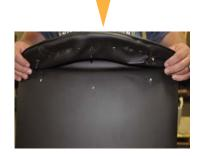
**EXECUTIVE:** The seat and the back are a one piece assembly made up of 3 wood substructures (1 inner back, 1 seat, 1 main substructure). The seat is fastened to the main substructure with 4 screws. Using the phillips head screwdriver, remove the 4 screws. If applicable, a filler plate is attached to the main substructure with plastic push in fasteners. Using the flat head screwdriver, pry away the filler plate.
