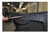
**EXECUTIVE:** The mesh upholstery is stapled to the inside of a plastic back frame piece. Remove the staples using the staple puller. Pull the mesh upholstery away from the plastic frame.
