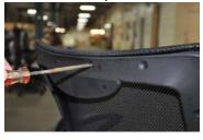
The mesh upholstery is stapled to the inside of a plastic back frame piece.
